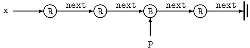
the relation  $x \langle \text{next.next} \rangle (\text{List:blue}) ? p$  is true, whereas the relation  $p \langle \text{next} * \rangle x$  is false. We allow the usual syntactic sugar, such as `true`, `!`, `=>`, `<>`, and `all`. Furthermore, the unary relation  $\langle \mathbf{R} \rangle c$  abbreviates  $c \langle \mathbf{R} \rangle c$ . Some examples of general formulas on stores are:
