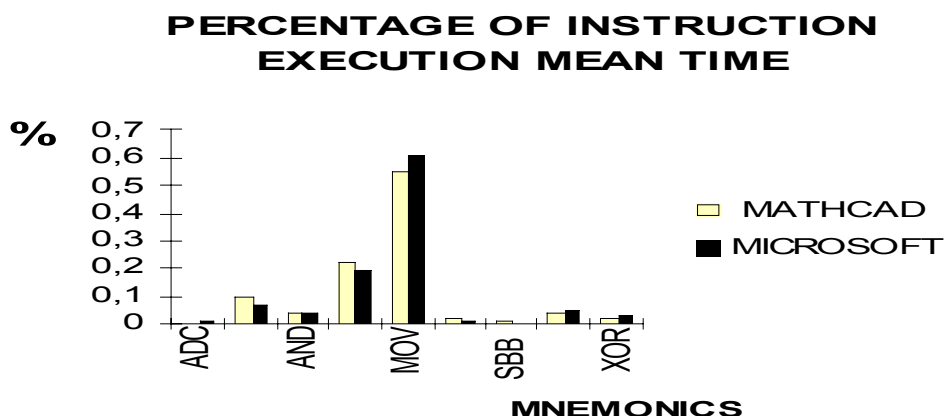
Fig. 1 Diagram of f_i \cdot \tau_i / \sum f_i \cdot \tau_i data for five upper (in terms of this percentage) x86 instructions emulated on the RISC platform.
