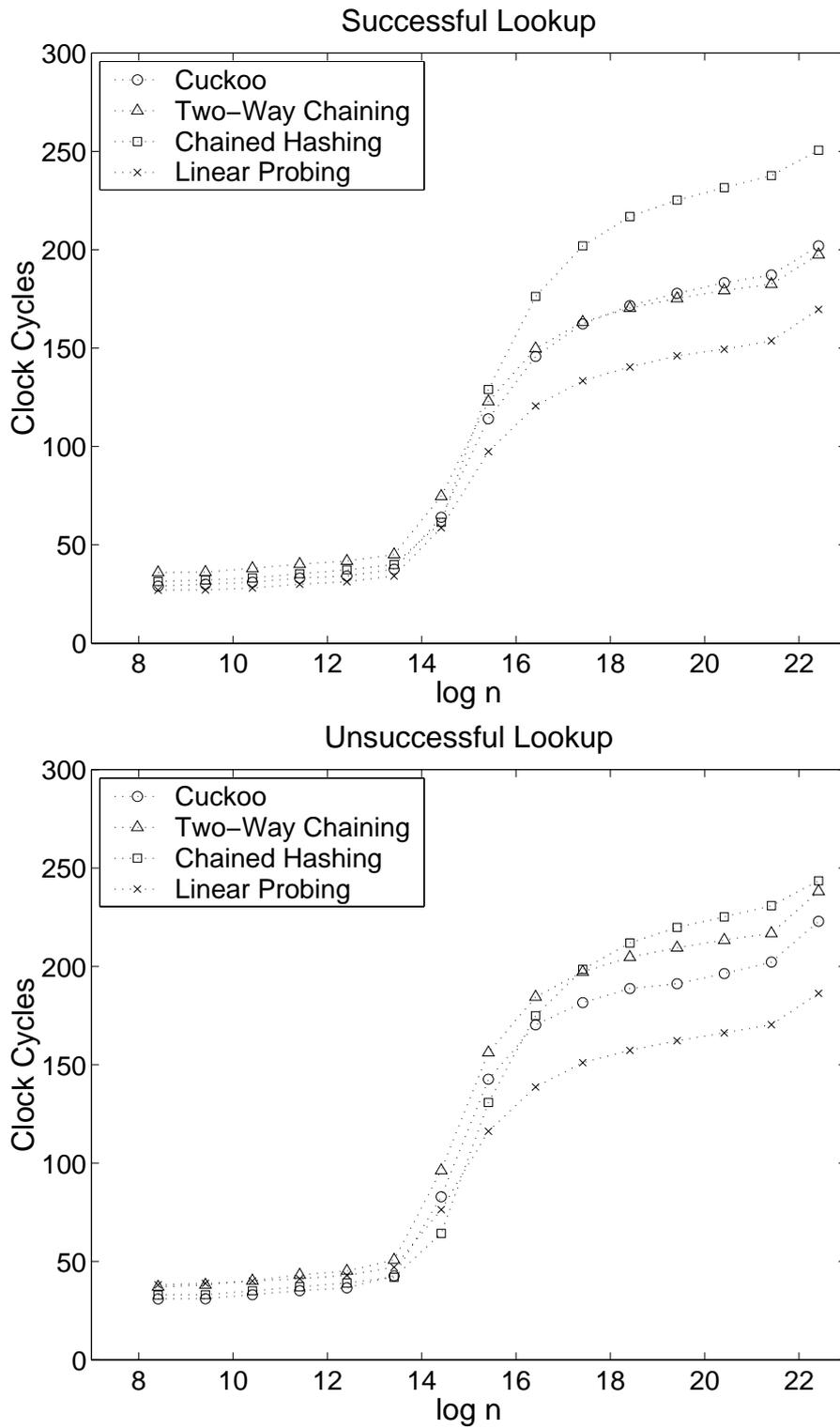
**Figure 4.3:** The average time per operation in equilibrium for load factor 1/3.
