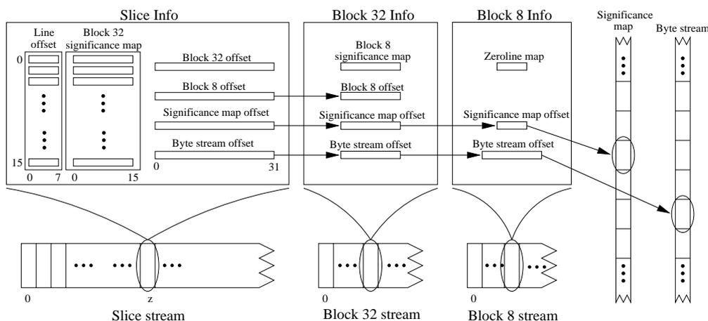
**Figure 7.3:** Data structure used for encoding significant wavelet coefficients.
