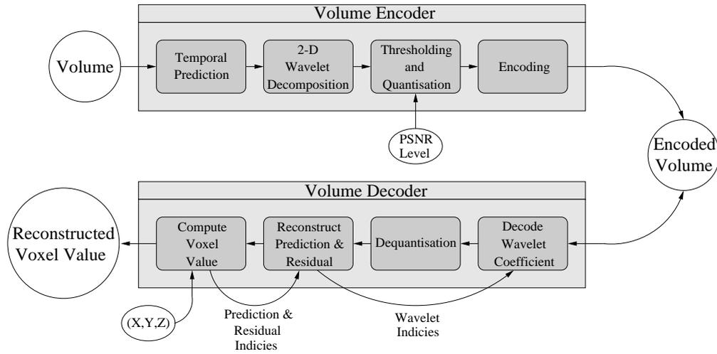
**Figure 7.1:** Overview of the encoder and the decoder.
