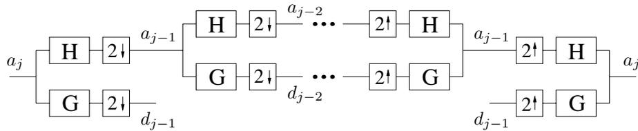
**Figure 2.1:** A 3-channel filter bank for computing a two level wavelet decomposition and its inverse.
