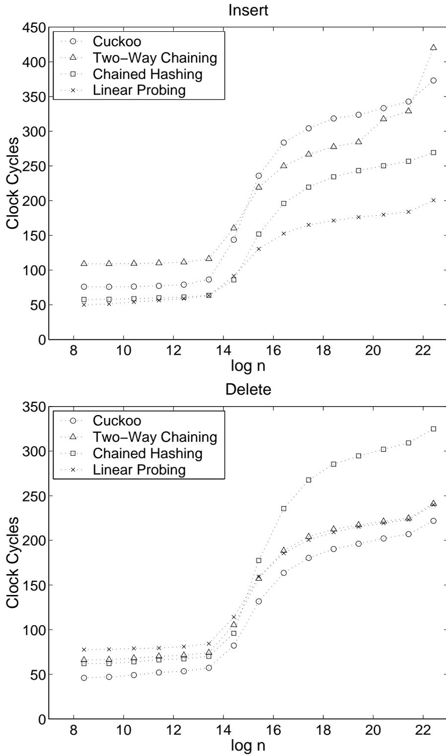
Figure 4.4: The average time per operation in equilibrium for load factor  $1/3$ .
