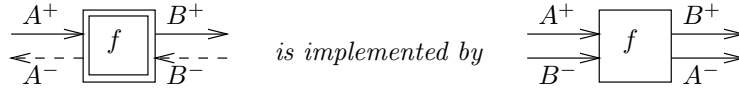
Figure 8.6: A process with bi-directional I/O implemented by an uni-directional process. Dotted lines indicate channels that play the opposite role in the higher-order model
